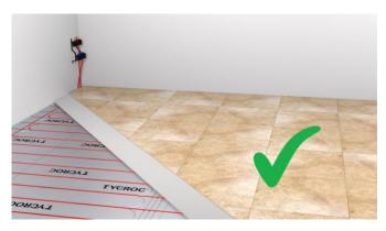
**IT IS PERMITTED** to install Tycroc UHP panels by the screwing method if the subsequent coating material will be installed floatingly!
