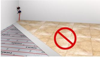
IT IS PERMITTED to use ceramic tiles or natural stones if Tycroc UHP panels themselves have been installed using bonding method!
