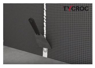
The gaps between building boards and corners should be covered with adhesive sealant, and also fastening dowels should be covered with Tycroc Premium FIX adhesive. Direct water contacted corners, cover additionally with waterproofing tape and —membrane.
