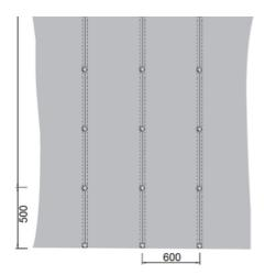
A) / B) Place building board on the floor and press it strongly against the surface, fixing the building board with suitable screws and metal washers 36x0,6 mm. Use screws that enter the underlying surface by at least 20 mm.
