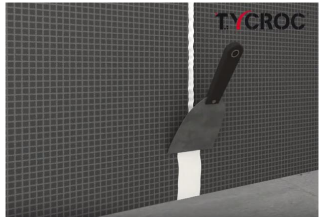
The gaps between building boards and corners should be covered with adhesive sealant, and also fastening washers should be covered with the help of a spittle. Direct water contacted corners, cover additionally with waterproofing tape and -membrane.
