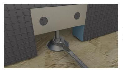
The bathboard can be fastened using the adjustable legs, raising the board firmly up to the bath edge. 13 mm spanner is suitable for adjusting.
