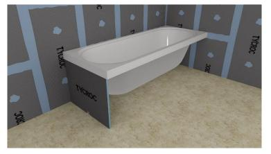
If necessary, cut the bathboards to the right size. Make sure that, apart from a Tycroc bathboard, there would also be space under the bath for ceramic tiles or natural stone to be used later. Apply Tycroc Premium Fix adhesive sealant to the upper edge of the bathboard, so that the edge would be continuously covered with adhesive sealant.
